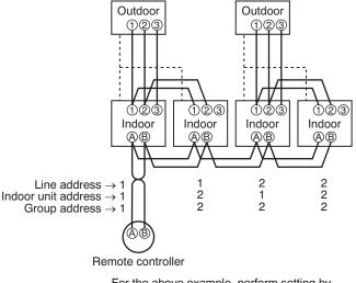
For the above example, perform setting by connecting singly the wired remote controller without remote controller inter-unit cable.
